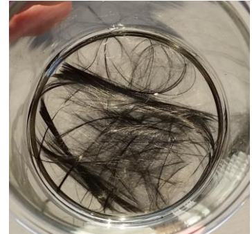
LYSAPUR PU30 quickly dissolves prepreg at 21°C
